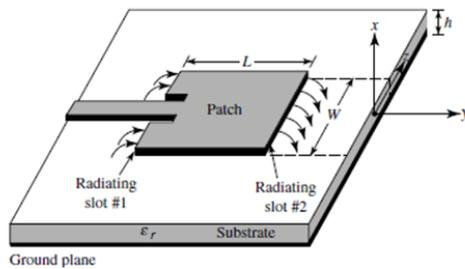
**Figure 2.** Model of Antenna Microstrip for Broadband Wireless Communication
