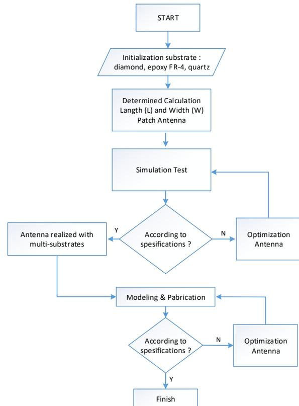
**Figure 1.** Flowchart of Multi-Substrate Microstrip Antenna Design using Quantitative Empirical Method
