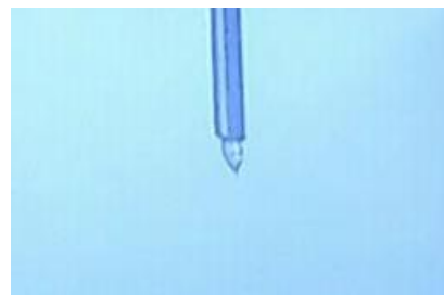
Figure 2. The Taylor Cone of Nylon-6 Solution
