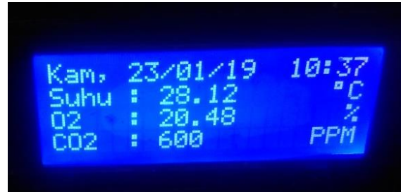
Figure 2. Display data to 20x4 Character LCD
